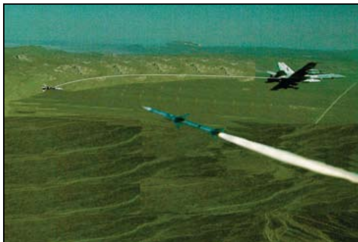
FIGURE 1 Photograph of a misdirected missile heading towards a decoy attached to a towline behind a military fighter aircraft.
