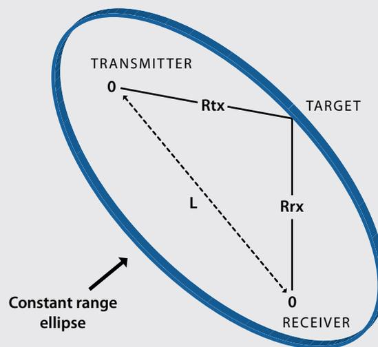
Note:  $R_{tx}$  = transmitter range to target;  $R_{rx}$  = receiver range to target;
