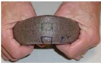
Figure 12: Foam Rod Failure
