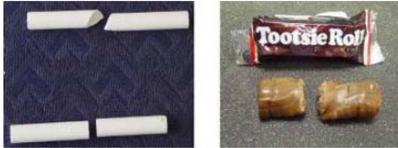
Figure 2: Failure modes of chalk in torsion (top) and bending (bottom) and Tootsie Roll in torsion.
