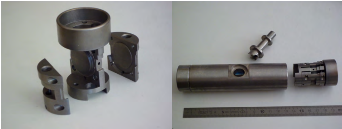
Fig.6 The endcap (left photo) is isolated from the main body of the electrode (right photo, center object) via a high-Q, about 400 pF capacitance consisting of 4 sapphire disks of thickness 0.2mm, diameter 25mm, to be on the (almost) same RF potential as the electrode, but to be biased to -2 kV DC.
