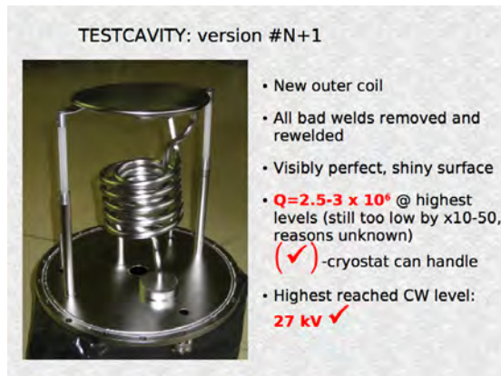
Fig.5 Superconducting test cavity (after many iterations) has now reached Q = 2.5 - 3 \times 10^6 and can sustain a peak-to-peak voltage of 27 kV.
