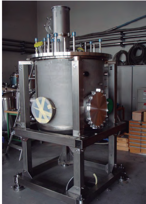
Fig.1 The cryostat for the Paul trap has been completed in the CERN Cryolab.
