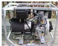
3.5kW Auxiliary Power Unit to support Asymmetric Threat Defeat JUONS
