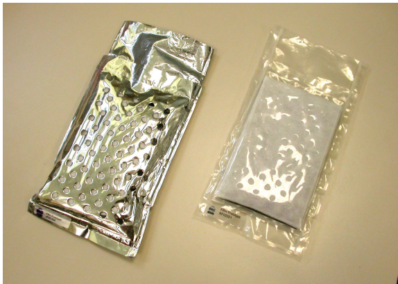
Figure 6. Prototypes of air-activated heaters using a 4-layer metalized film (left) and Curlam ® Grade 1834-K protective packaging film (right)
