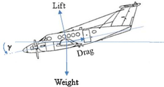
Figure C-1. Forces in a Stabilized, Zero-Thrust Descent
