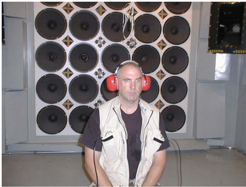
Figure 6: AFRL’s high intensity reverberation chamber – 142 dB max overall sound pressure level capability
