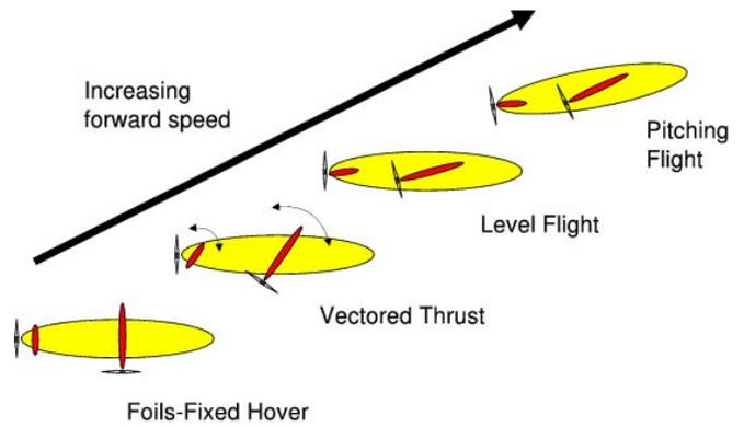
Fig. 11. *Nereus*'s depth and pitch control modes [18]. Lift-dominated low angle of attack flight modes will enable efficient operation at high speeds. Thruster-dominated high-angle of attack hover modes will produce the climb angles necessary to negotiate steep terrain at low speeds. Foils-fixed hover and the two flight modes were demonstrated successfully in the recent sea trials.
