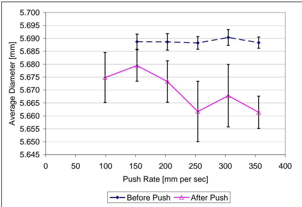
Figure 16. Plot of the average diameter before and after the push test.
