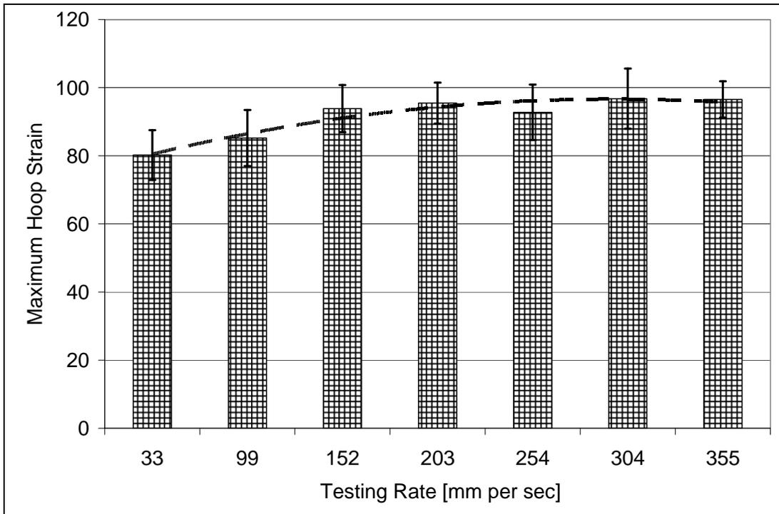
Figure 15. Plot of the maximum hoop strain on the OD of the barrel vs. displacement rate.
