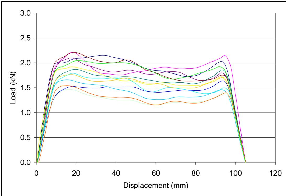
Figure 10. Load vs. displacement for 254-mm/s displacement rate.
