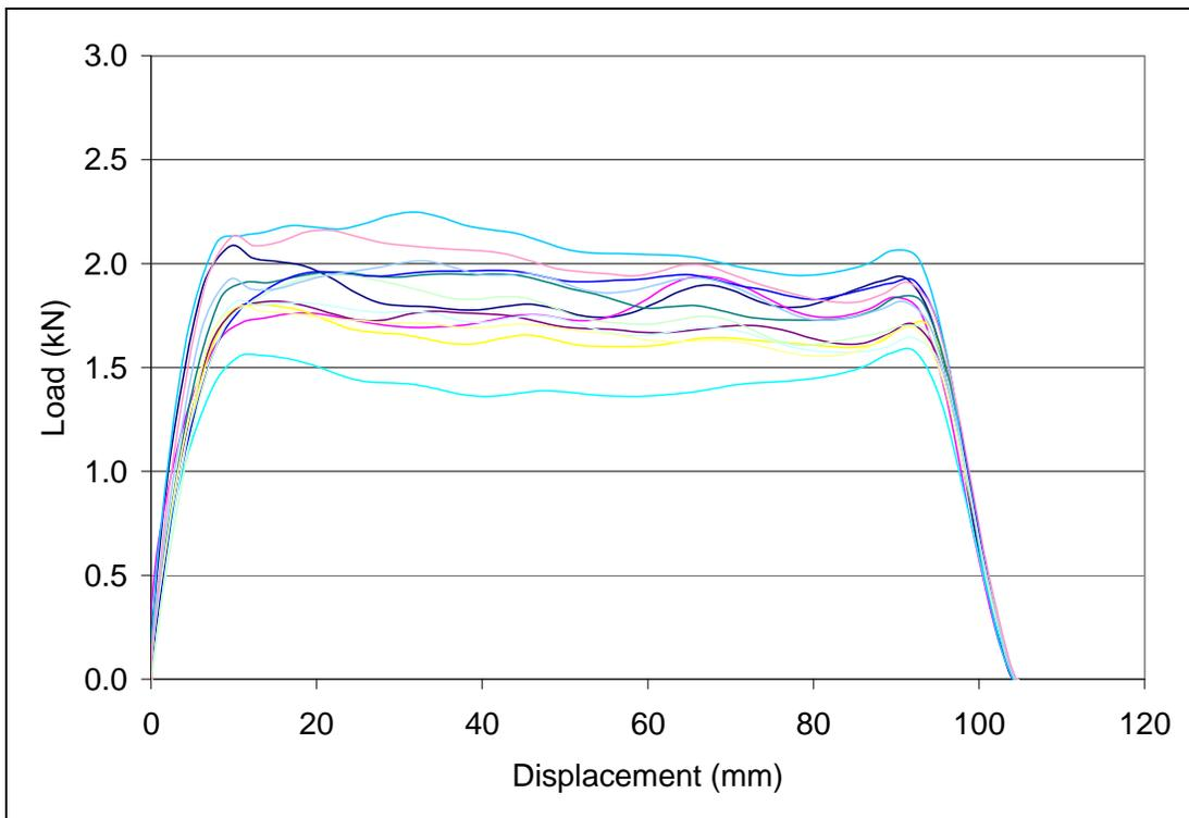
Figure 11. Load vs. displacement for 304-mm/s displacement rate.
