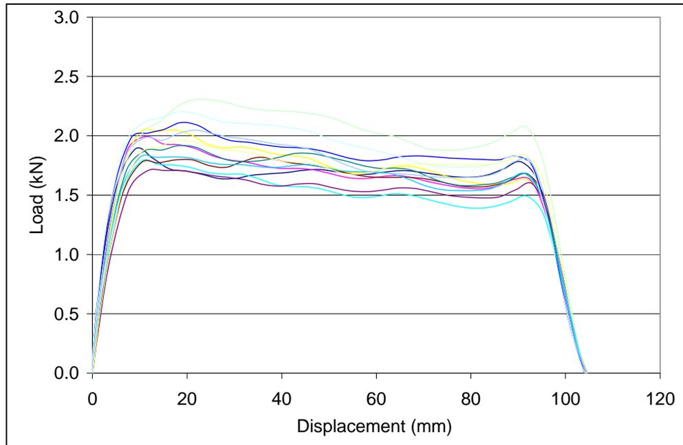
Figure 12. Load vs. displacement for 355-mm/s displacement rate.
