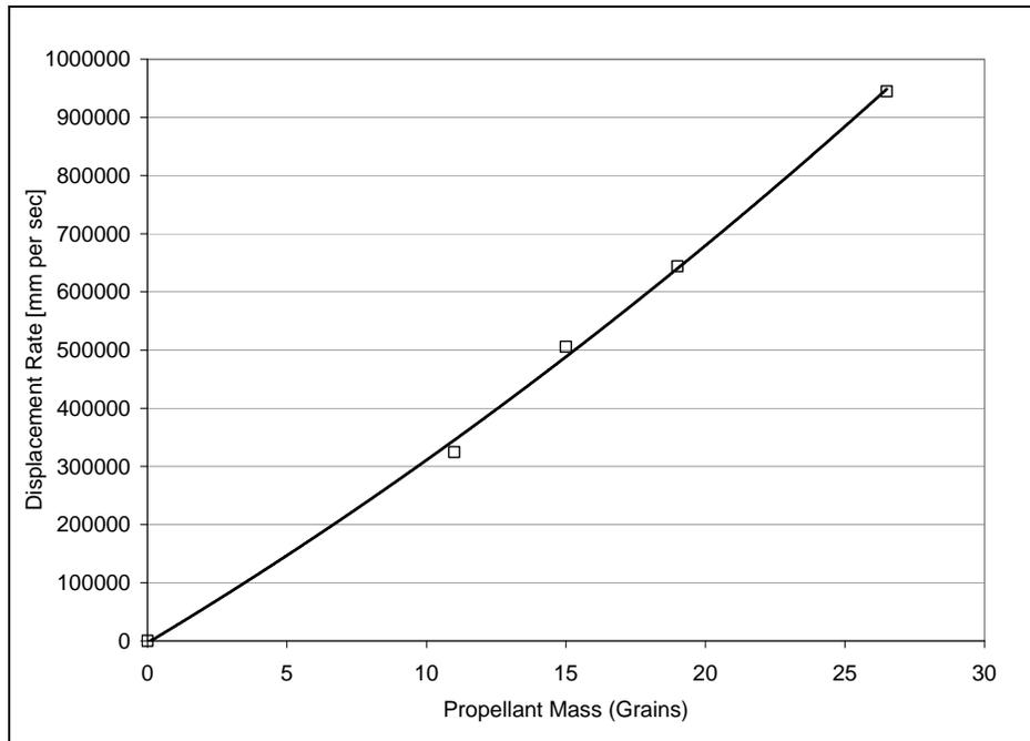
Figure 5. Plot of the displacement rate, at the muzzle, vs. propellant mass for WC844 and the M855 cartridge/projectile fired from an M16A2.
