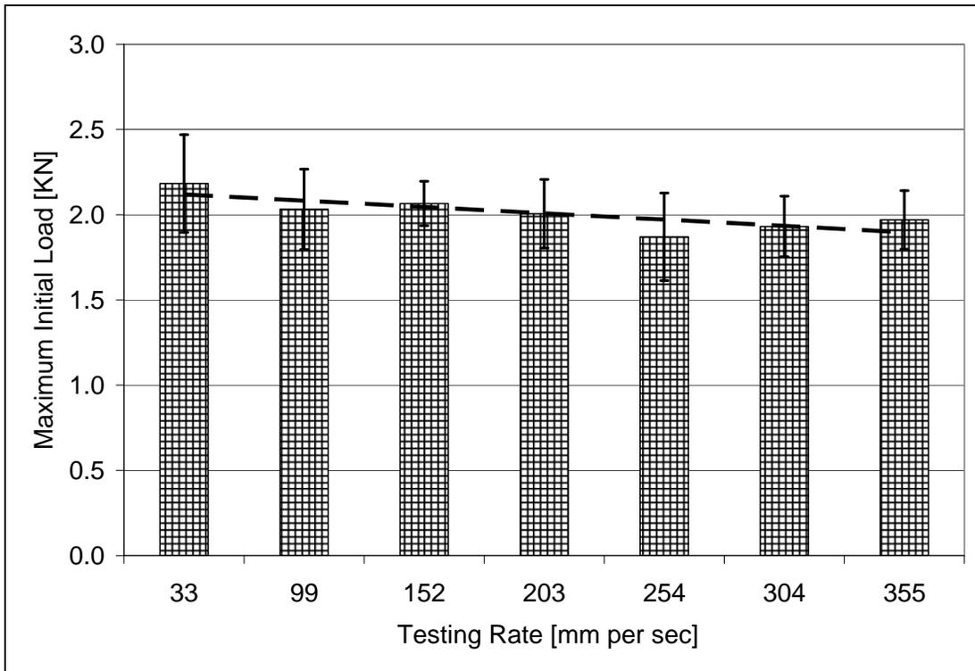
Figure 13. Plot of the average maximum initial load vs. displacement rate.
