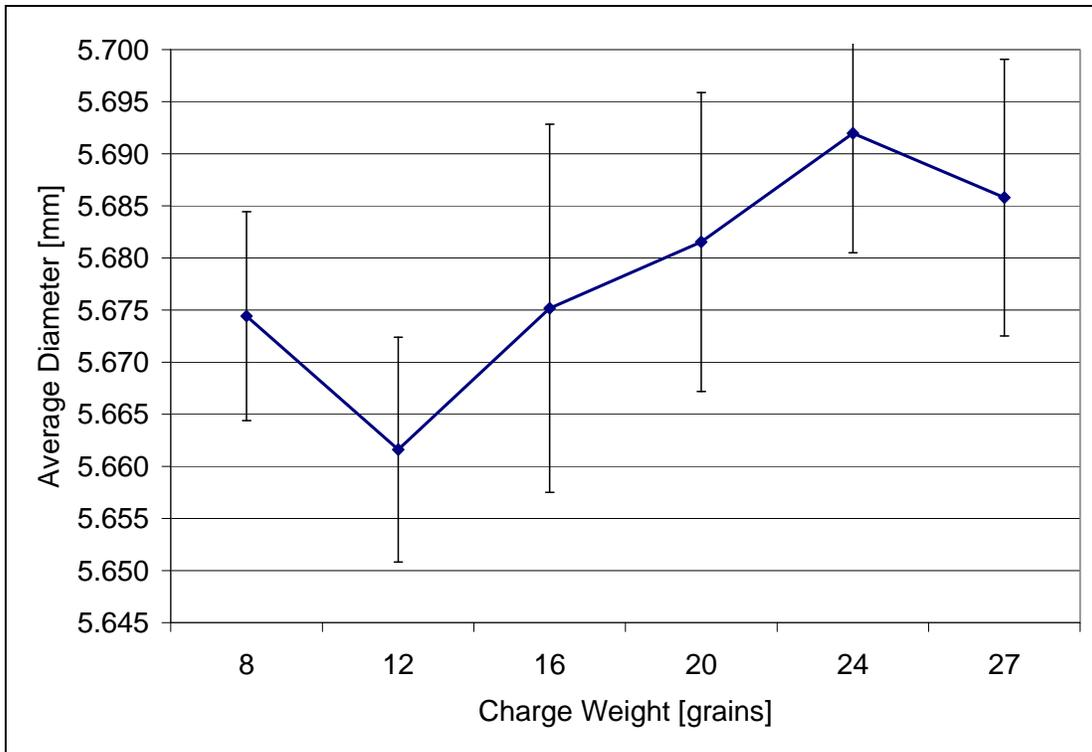
Figure 18. Plot of the average diameter vs. the charge weight for soft recovered projectiles.
