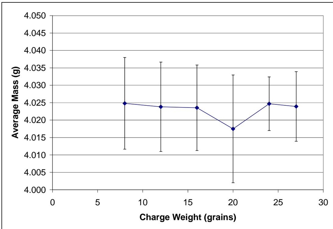
Figure 19. Plot of the average mass after soft recover vs. charge weight.
