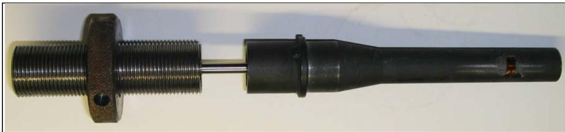
Figure 4. Image of the push rod, rod adaptor, and the sectioned M16A2 barrel.
