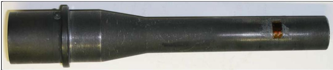
Figure 3. Section of a M16A2 barrel used for push testing.
