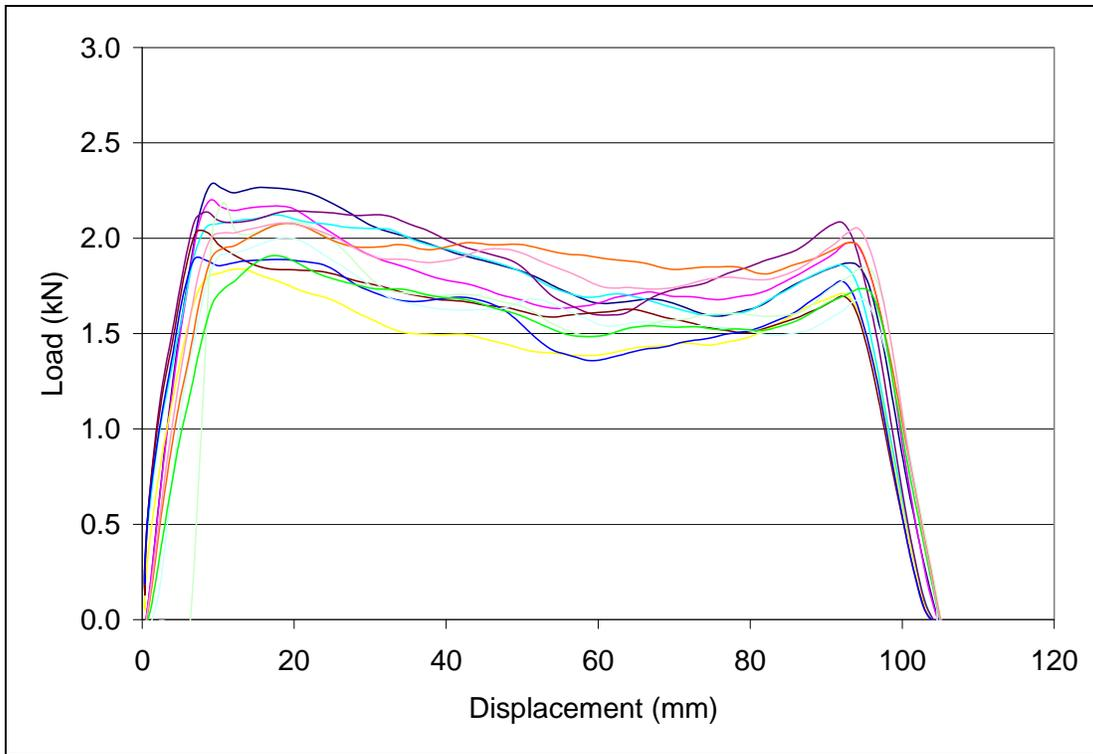
Figure 8. Load vs. displacement for 152-mm/s displacement rate.
