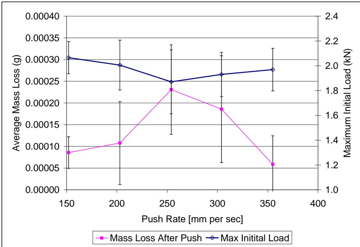
Figure 20. Plot showing the relation between the average mass loss and maximum initial load vs. push rate.
