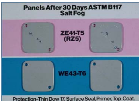
Figure 5. Proper alloy selection and adequate engineering solutions could potentially mitigate Mg alloys corrosion. Photograph depicting the improved corrosion resistance of Elektron WE43 vs. ZE41.
