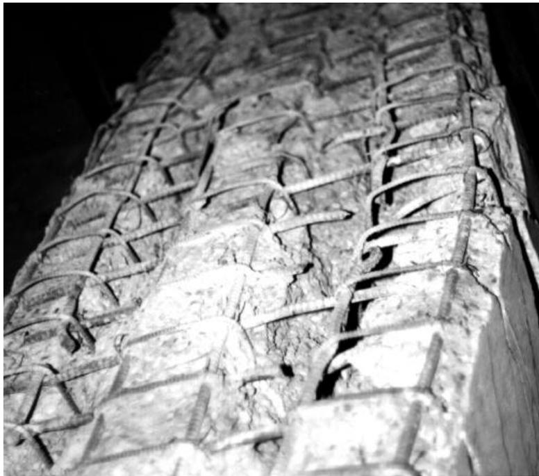
Figure 1. Pictures of fragment damage of a reinforced concrete slab caused by a cased munition.
