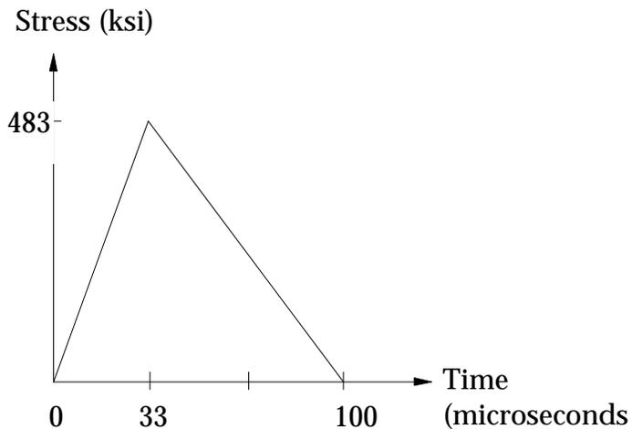
Figure 6. Pressure history equivalent of fragment loading.
