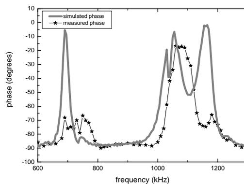
Figure 19: Phase spectra for a 2 mm Pz27/1.6 mm Al/2 mm Pz27 AEF configuration
