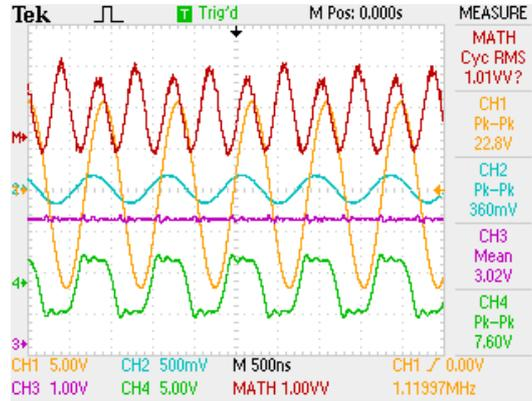
Figure 17: Oscilloscope screen capture showing four example voltage traces from the aluminium plate AEF experiment. Channel locations are indicated in Figure 8b: Ch1= $V(in)$ , Ch2= $I(R2)$ , Ch3= $V(out)$  across  $30\ \Omega$ , Ch4= $voltage$  across the receive piezo
