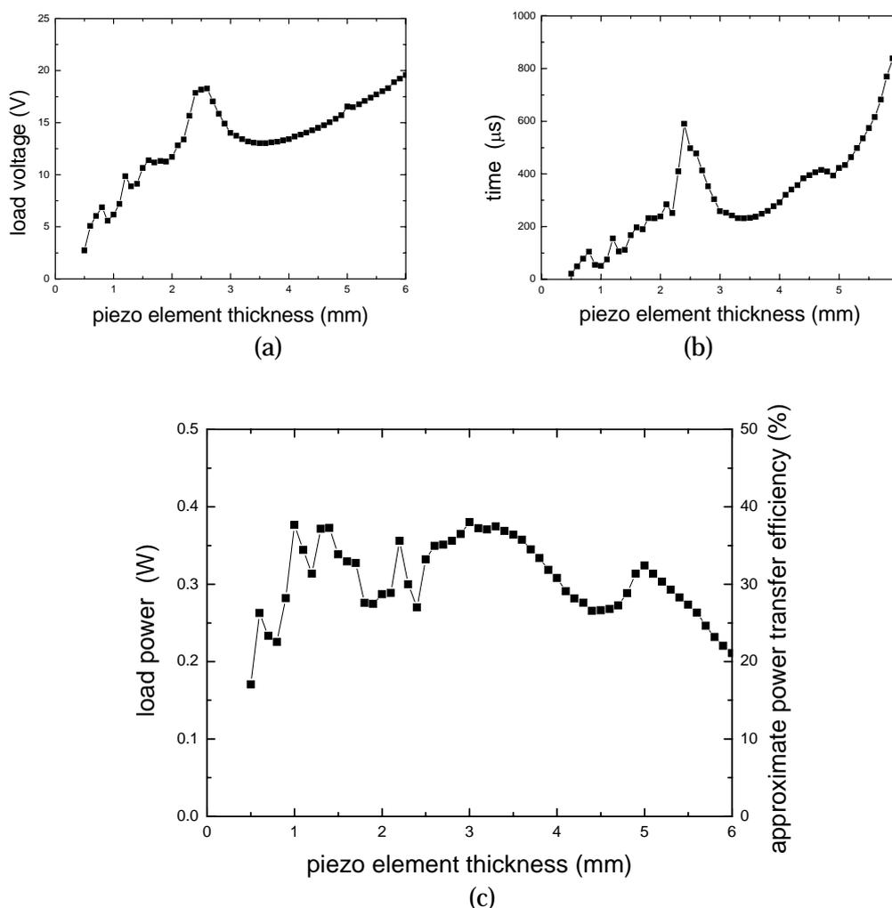
Figure 22: Modelled results for an AEF system for a 1.6 mm thick Al plate, where the PZT element thickness is varied: (a) 90% of steady state load voltage, (b) time taken to reach 90% of steady state load voltage, and (c) load power as a function of varying Pz27 thickness
