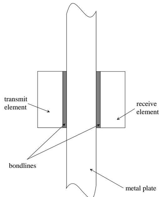
Figure 3: Schematic showing an AEF configuration in cross-section
