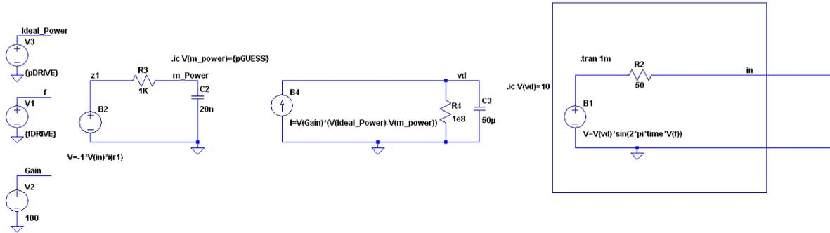
Figure 6: Schematic of the constant power source
