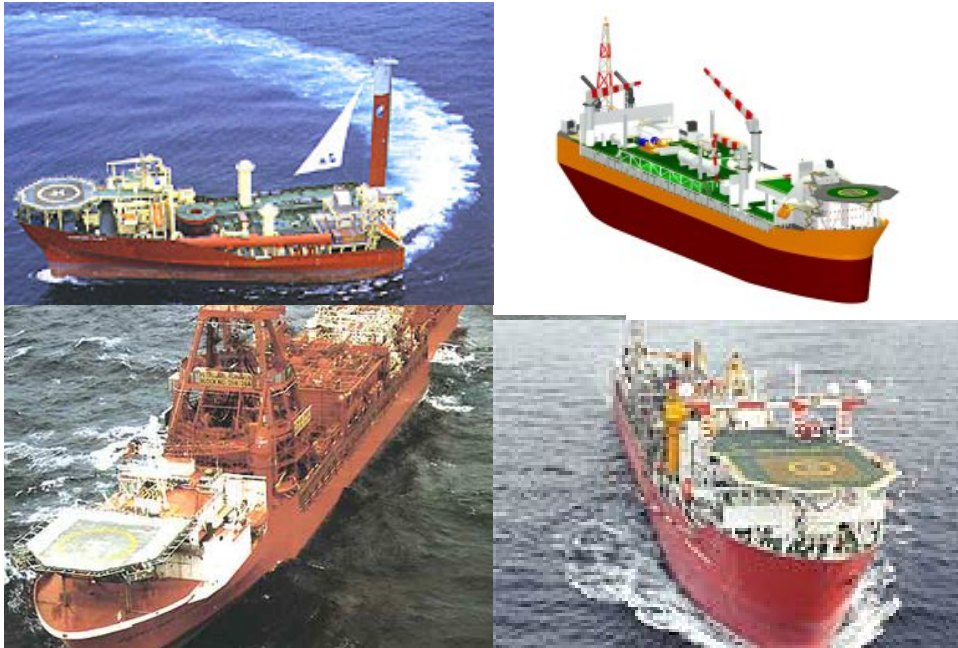
Figure 9 - Examples of Forward Helicopter Decks on FPSOs
