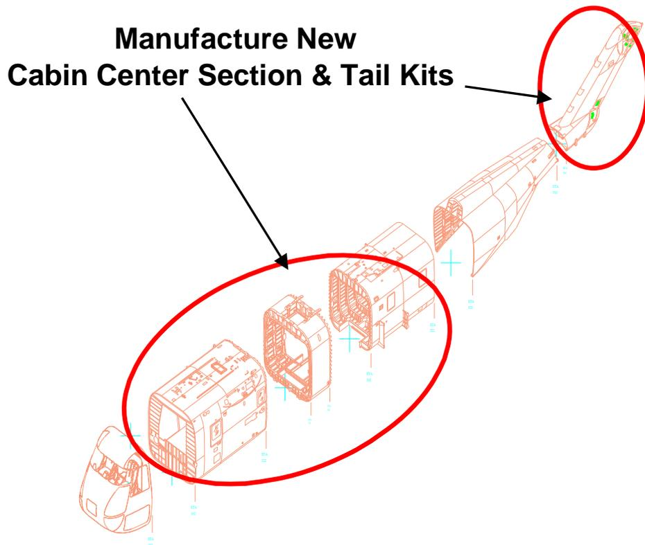
**Figure 7. Service Life Extension Airframe Modifications**
