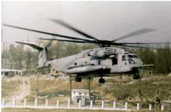
**Primary function:** Transportation of heavy equipment and supplies during the ship-to-shore movement of an amphibious assault and during subsequent operations ashore.
