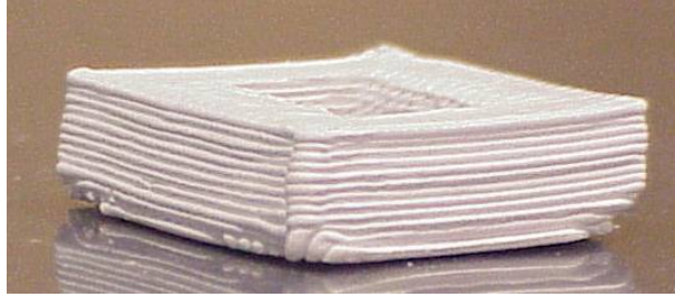
Figure 16: Side view for slanted part fabricated from starting/stopping extrusion.
