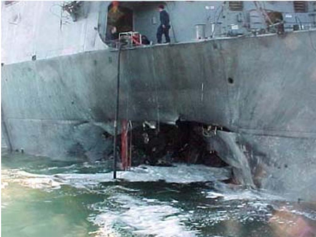
Figure 1. Damage to USS Cole from FIAC attack
