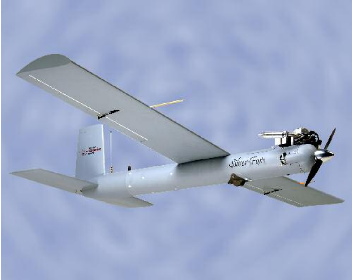
Figure 3: UAV (Silver Fox developed by Advanced Ceramics Research – photo used by permission) weighing twenty-seven pounds. This UAV is capable of thirty-five knots average speed, eight hours in flight mission time, 12,000 foot service ceiling, and a five pound payload. The UAV is inaudible at 700 feet and almost undetectable to the naked eye at 1,500 feet. It can also be launched from any site utilizing a portable launcher and requires no runway for recovery.
