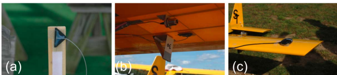
Fig. 2. (a) A custom-made dipole antenna installed on a ground node; (b) a dipole antenna installed beneath a UAV wing (inside a cardboard bracket); and (c) a GPS receiver mounted on a UAV wing.
