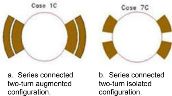
Figure 8. Two basic configurations considered for railgun design.
