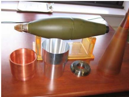
Fig. 1. Mortar round is adapted to the EM launch environment with a conformal armature tail kit.
