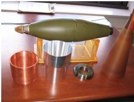
Fig. 1. Mortar round is adapted to the EM launch environment with a conformal armature tail kit.
