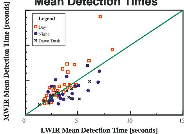
Figure 5. MWIR vs LWIR mean detection time for conventional targets in rural environment.
