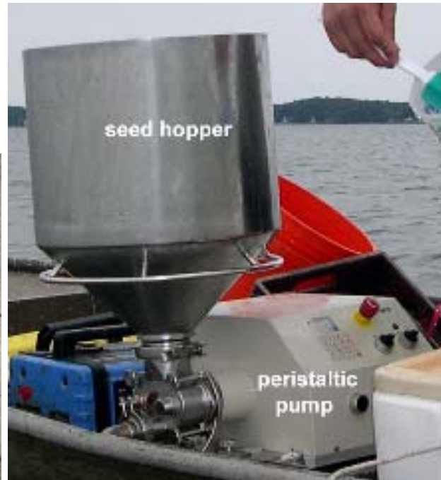
Figure 3. Seed/gel pumping mechanism.
