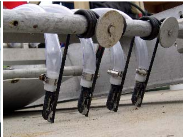
Figure 5. Spring-loaded seed injecting nozzles.
