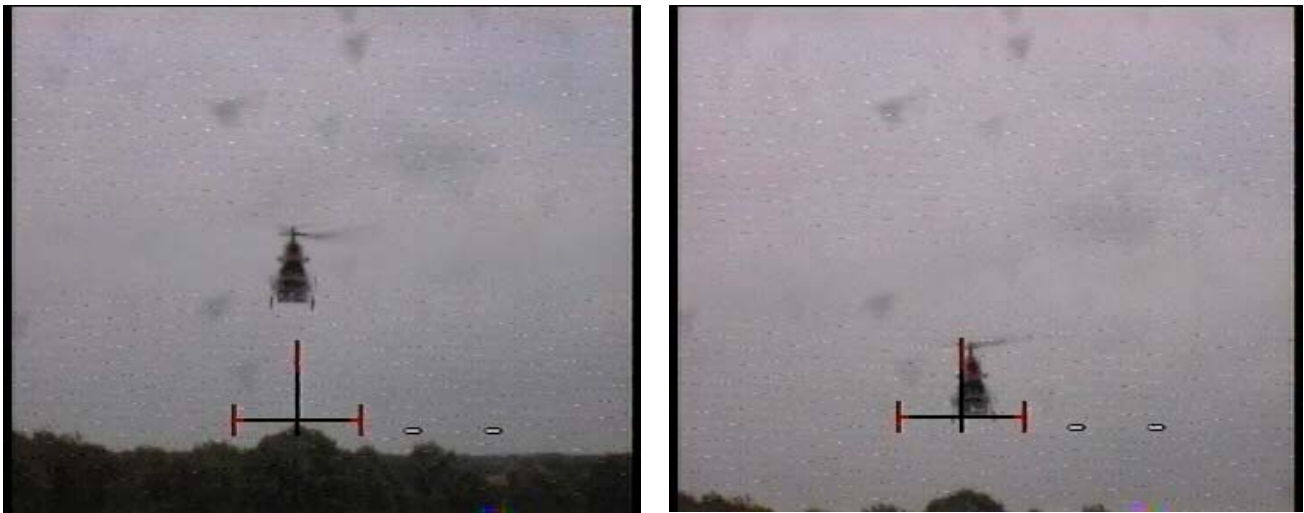
Figure 8 – Decking views recorded by the camera onboard the platform physical simulator (a representation of the platform position and width is inserted in images)
