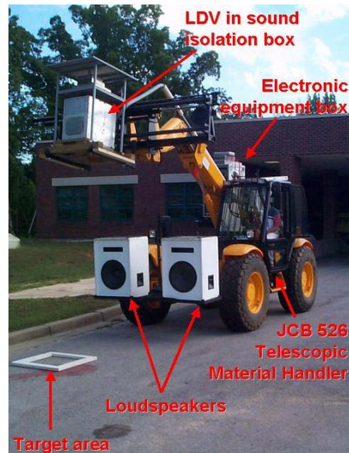
**Figure 2.** Photograph of the laser Doppler vibrometer-based acoustic-to-seismic landmine detection system.
