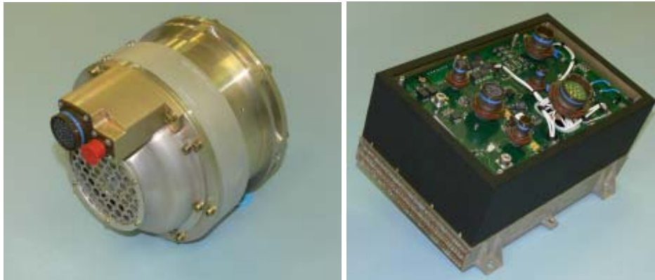
Figure 7: 270 VDC Starter Generator with Generator Control Unit
