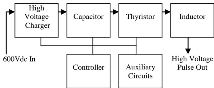
Fig. 4. Block diagram of major ETIPPS subsystems.
