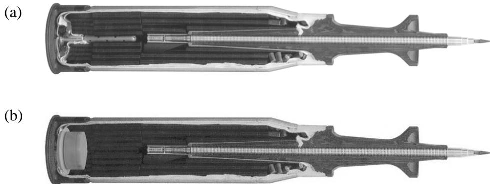
**Fig. 1. Conventional 120 mm M829A2 round: (a) with M129 primer; (b) with coaxial plasma injector.**
