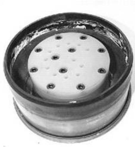
**Fig. 8. Coaxial Basepad injector and case base**
