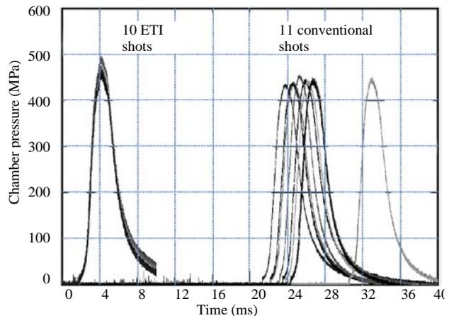
**Fig. 2. 11 conventional gunshot pressure traces (at right) and 10 ETC pressure traces (at left), demonstrating the repeatability of ETC versus the relatively random initiation obtained with conventional ignition.**
