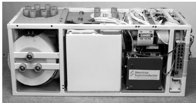
**Fig. 6. Photo of ETIPPS I, showing the General Atomics high energy density capacitor (white module in center of system).**
