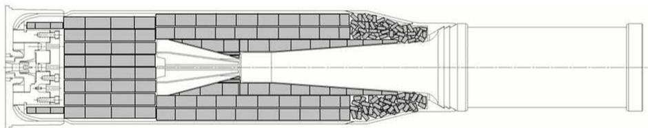
**Fig. 9. Coaxial Basepad injector in M829A2 slug round**
