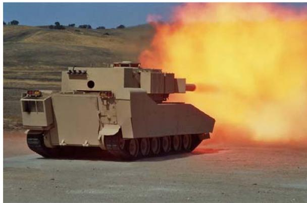
**Fig. 11. Lightning Bolt firing ETC modified M829A2 with ETIPPS II mounted on back of turret.**
