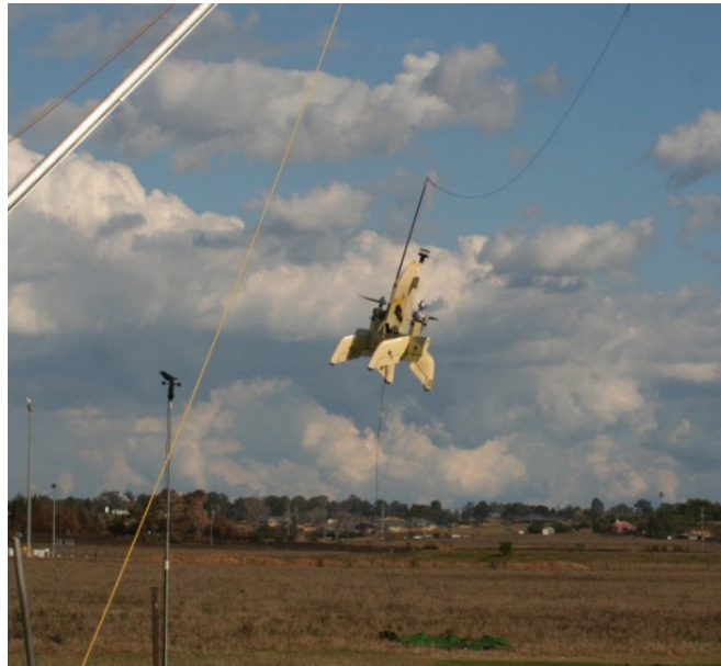
Figure 5: T-Wing flying autonomously on tether test-rig using MPC controllers designed by P. Anderson. (Note Ultrasonic Wind-sensor on nose).
