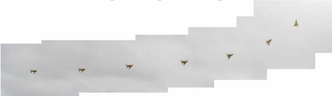
Figure 3: T-Wing horizontal to vertical (H2V) transition from, (made from multiple still frames shot in 0.3 second increments by Canon digital still camera)
