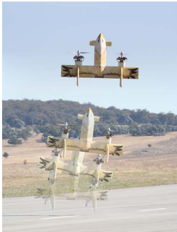
Figure 1: T-Wing autonomous takeoff, (taken from multiple frames shot at 0.33 second intervals with Canon Digital still camera)
