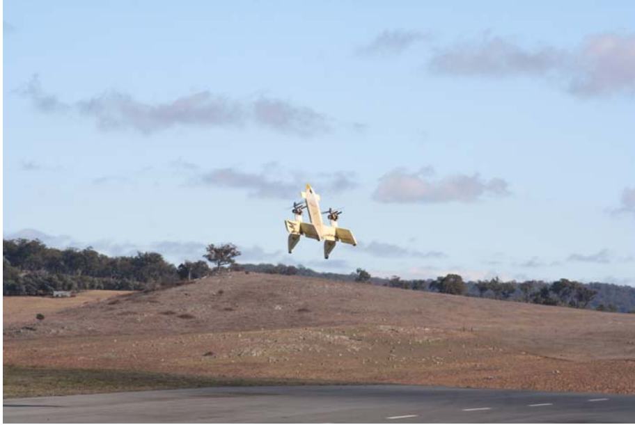
Figure 4: T-Wing landing while tilting into wind
