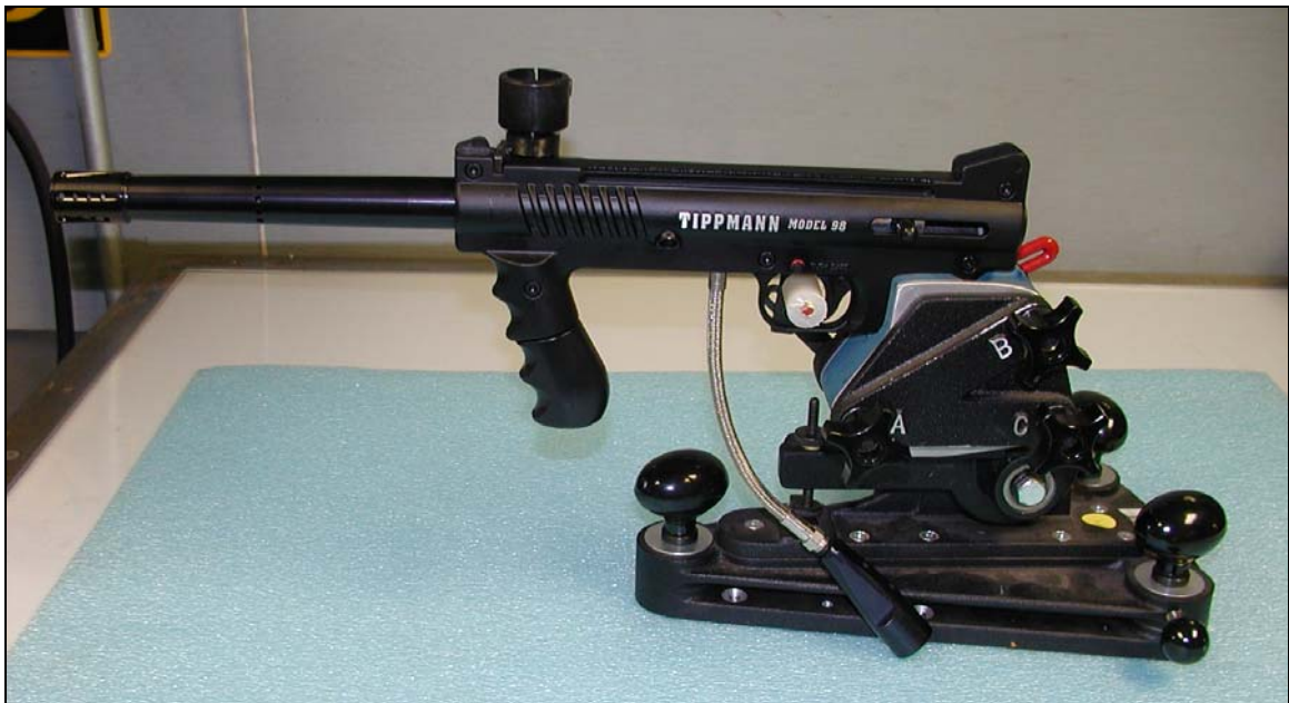
Figure 2. Firing setup for paintball testing.
