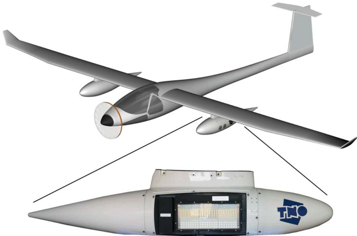
Figure 2: Example of a Motor glider, the Stemme S8. A mock-up of a SAR inside the pod is shown in the insert.
