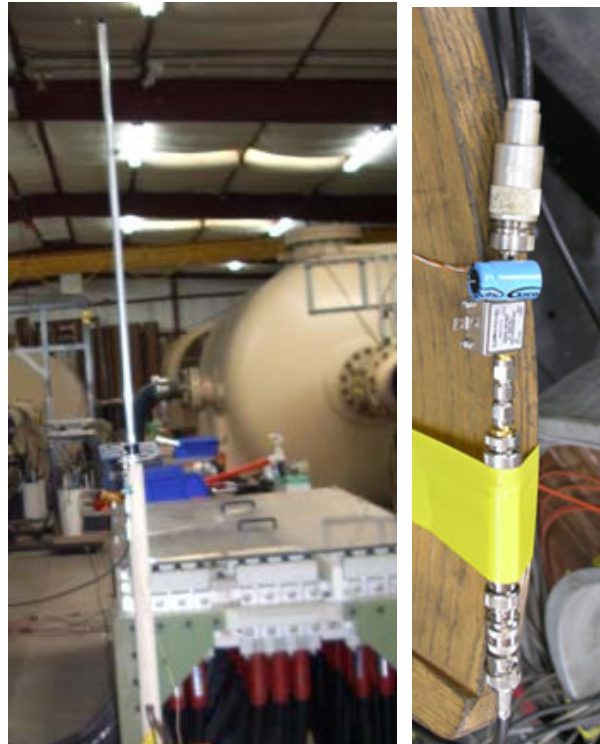
Figure 3. Antenna used to measure broad band RF radiation present during the tests. The signal is directly applied to a 100 MHz high-pass filter and 20 dB broadband amplifier (close-up at the right) before transmission via RG-8 coax to the digital oscilloscope.
