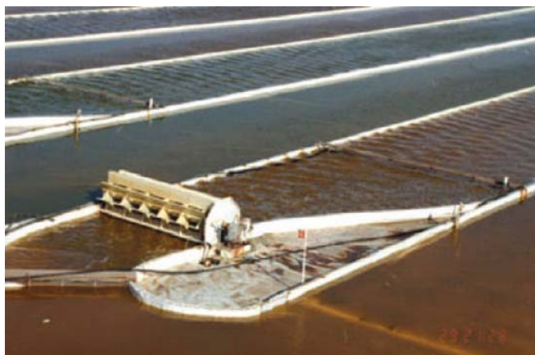
Figure E-1. Raceway Pond System in Israel Growing Microalgae
