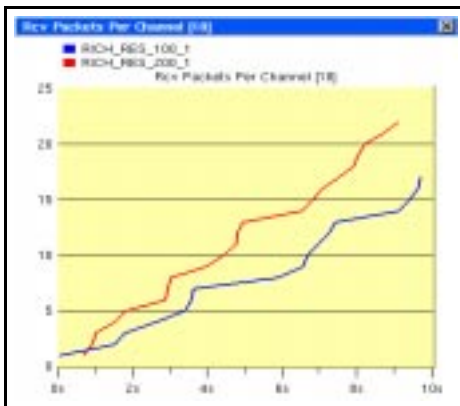
Fig. 7. Difference between an aggregate arrival rate that is less and more than the available channel bandwidth
