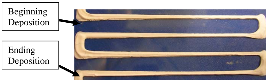
Figure 2: Deposition lines using constant ram velocity ( v = 0.5 \mu\text{m/s} ).
