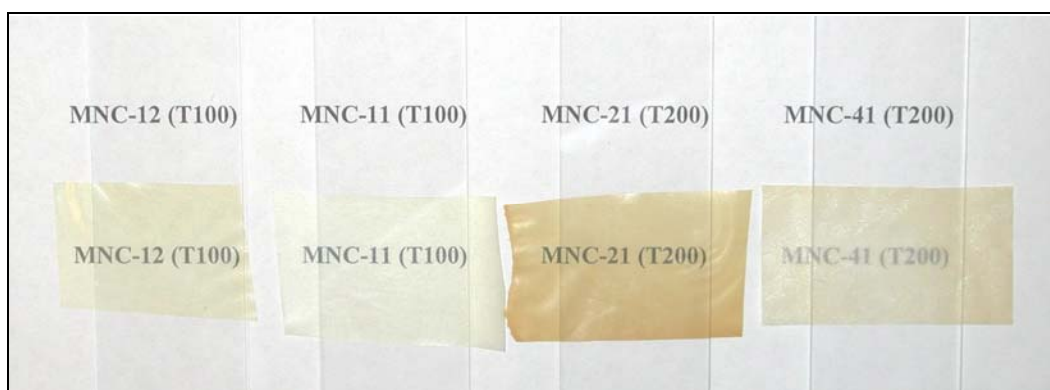
Figure 4. Comparison of optical clarity of selected MNC membranes. (Membranes are weighed down with glass slides.)
