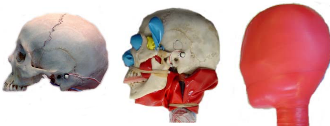
Figure 2. Creare Head Simulator. Left: dry skull with accelerometers mounted on the mastoid bones and on the interior temporal bones. Center: jaw added and organs simulated by latex balloons filled with silicone. Right: tissue simulated by silicone, muscle tension by elastic tape, skin simulated by balloons, remaining cavities filled with silicone oil to simulate cerebrospinal fluid.
