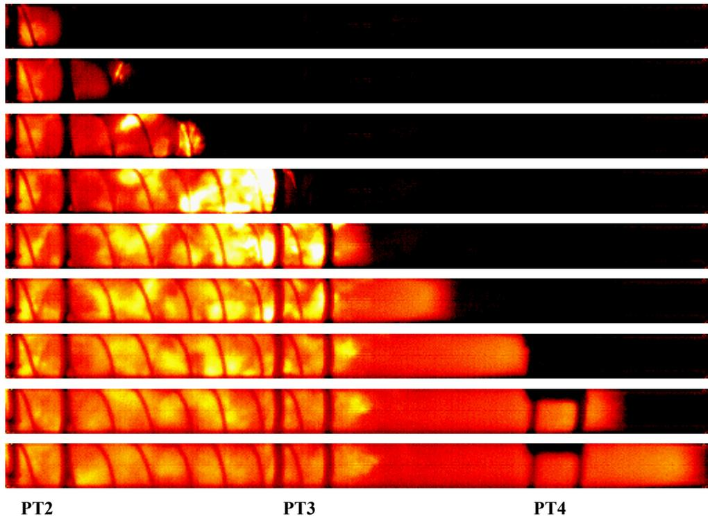
Fig. 5. Image sequence showing DDT initiated by a Shchelkin spiral with pitch of 1 tube diameter and length of 9.5 tube diameters. Images are spaced  $50 \mu\text{s}$  apart in time and begin  $5 \mu\text{s}$  after PT2 is triggered. Equivalence ratio is 1.0. Pressure transducer locations are labeled as PT2 to PT4.
