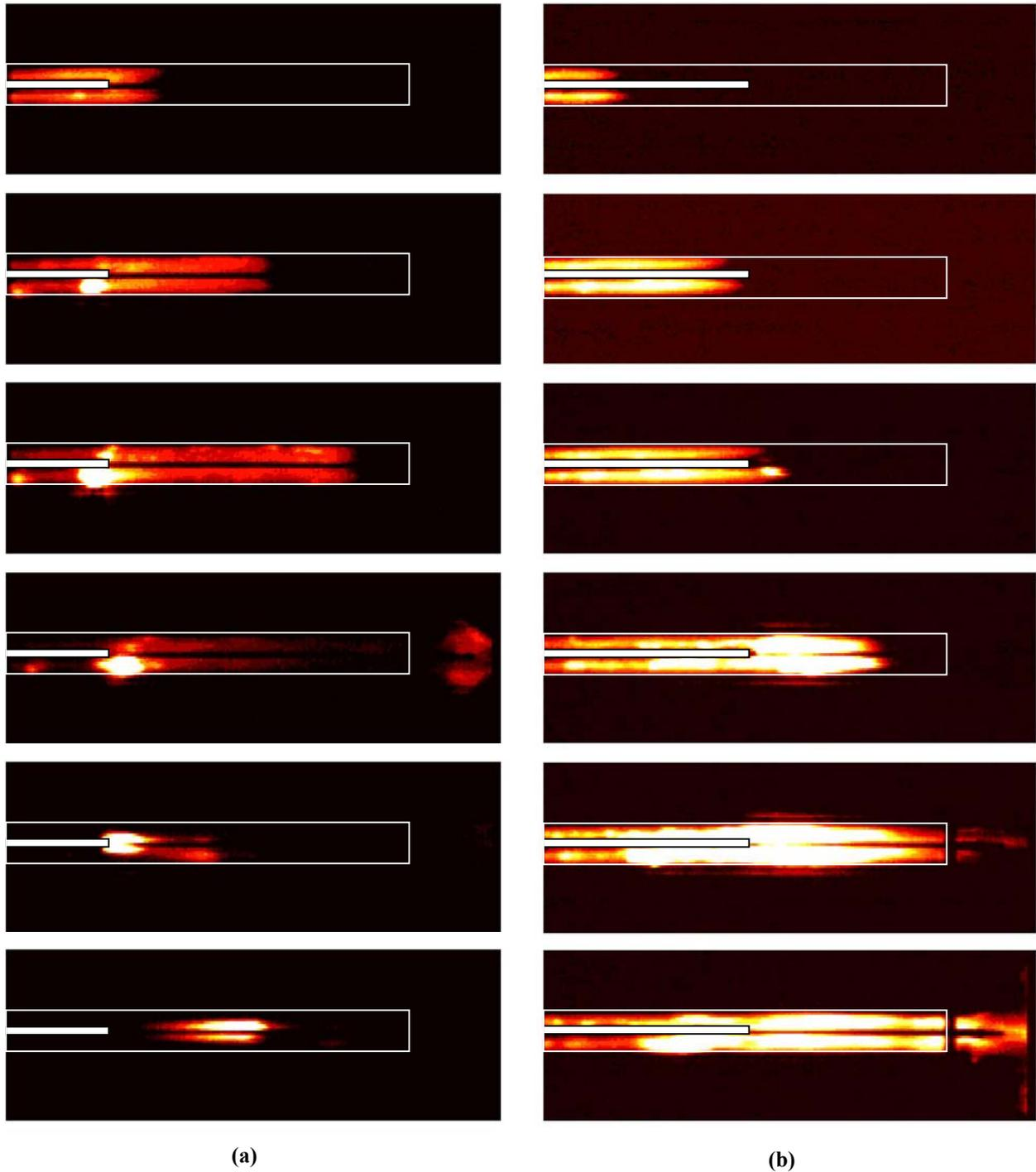
**Fig. 10. Image sequence showing co-annular tube DDT enhancement geometry with tube length of (a) 2.5 tube diameters and (b) 6 tube diameters. Equivalence ratio is 1.0. Maximum velocity of 520 m/s achieved for (b). Outlines of main and inner PDE tubes shown in white.**
