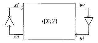
Figure 1: A one-place buffer and its interface
