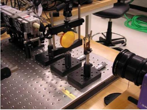
Figure 7. Schematic diagram of setup for measurement of THz beam diameter as obtained by dual lens system. The figure shows the position of the laser (upper left), plano concave lens, plano convex lens (large orange disk) and the thermal imaging camera (black lens cover at lower right).
