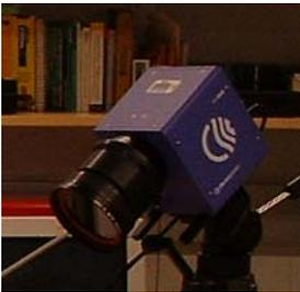
Figure 4. Side view of 320 x 240 pixel thermal imaging camera (Electrophysics PV320L2) used for THz imaging.
