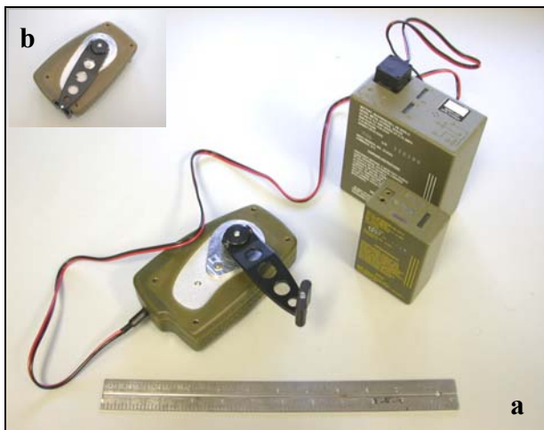
Figure 2. (a) Palm Power unit connected to a BB-390 battery. BB-2847 also shown. (b) Palm Power with hand crank stowed.
