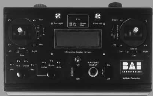
BAI's Flight Controller features all air vehicle command functions arranged for optimum ergonomics. A back-lit LCD displays mission programming data.
