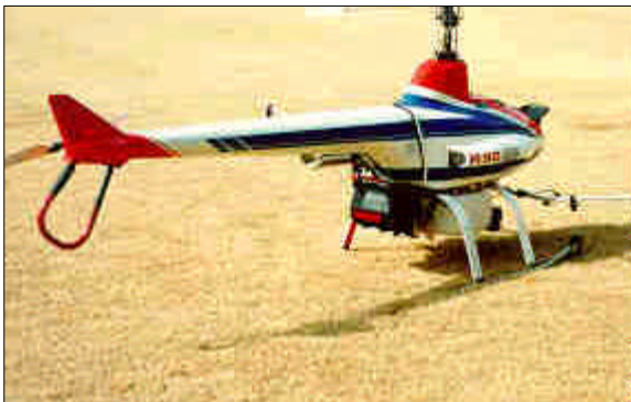
Fig.3 R50 Equipped with YOSS -Altitude Control Device
