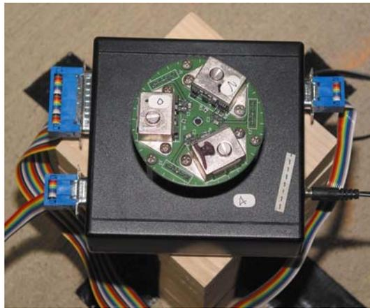
*Figure 2:BAE radar showing three emitter/detector pairs*
