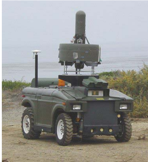
Figure 4. MDARS-E with Allied Aerospace's 29" iSTAR UAV and First Generation Launch Fixture
