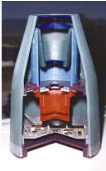
Figure 6. Cutaway of a DAMASK Seeker 6
