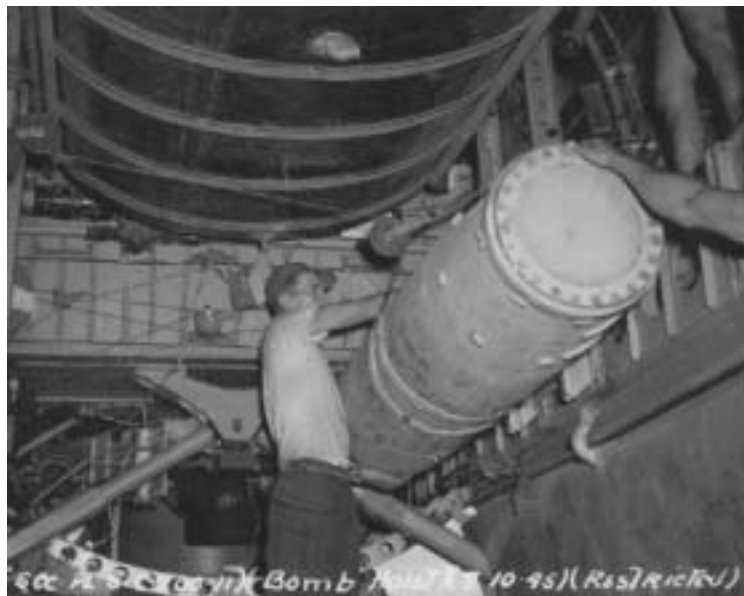
A 2000-pound MK-25 mine is loaded in a B-29's bomb bay. Photo 6
