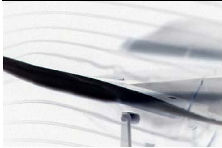
Figure 35. Flow Separation, V=2.0 m/s, 31 Hz, SM
