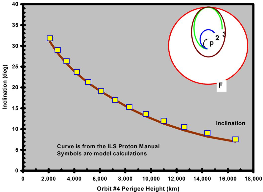
*Figure 4 Model calculation of the inclination of the high-energy transfer orbit as a function of its perigee height. The curve is from the ILS Proton Systems Manual. The points are the model calculations, which agree to within 1° of the rigorously derived and published values.*
