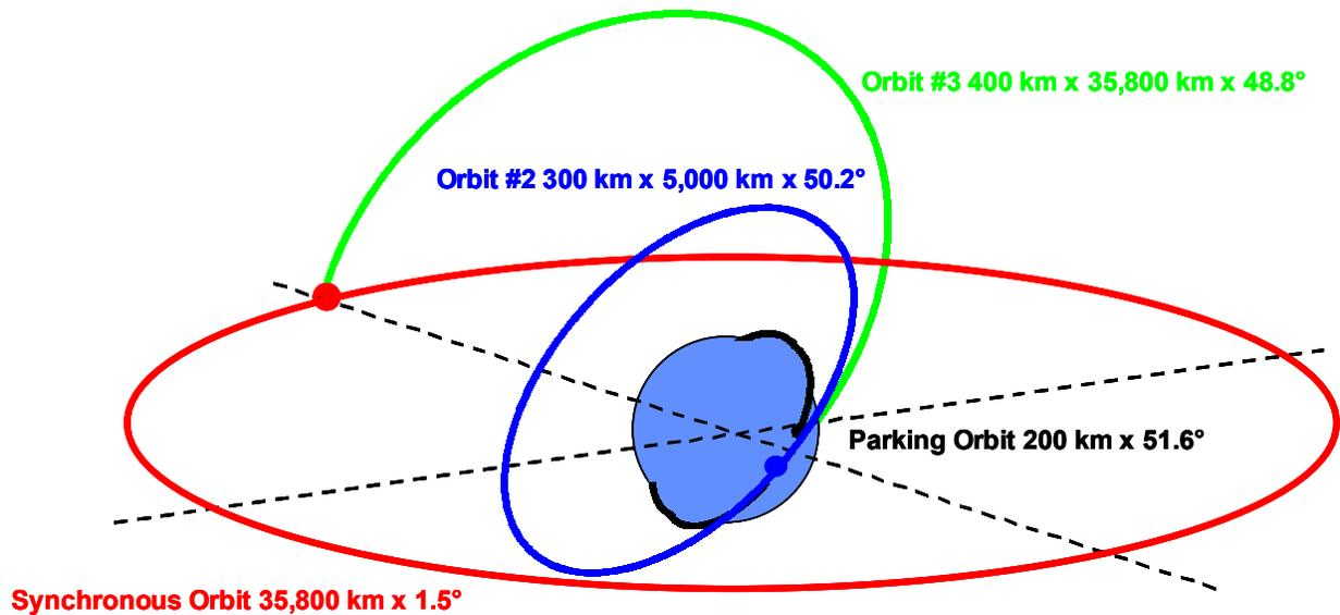
Figure 6 3-D representation of the Gorizont 45 launch
