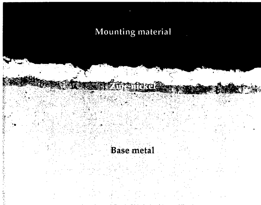
Figure 6. Cross section of the zinc-nickel-tin coating showing two distinct layers. Note the cracked zinc-nickel base coat and the structure within the tin topcoat (magnification 400 \times ).
