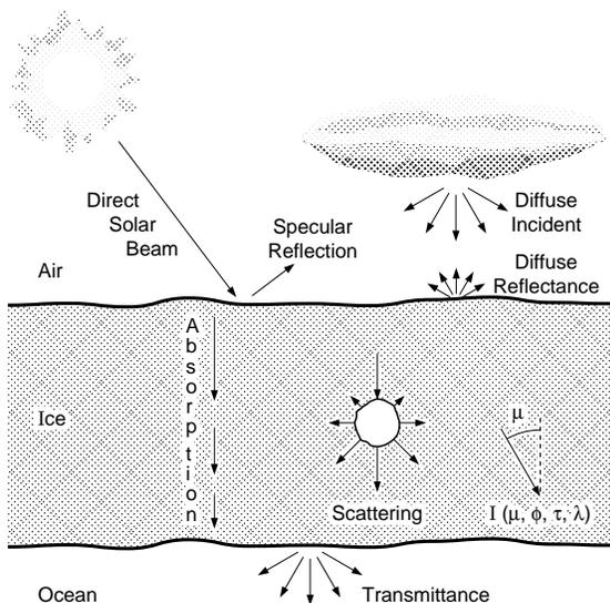
Figure 4. Schematic of radiative transfer in sea ice.
