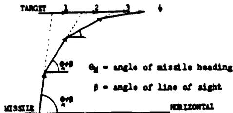
(b) Pursuit. Lead or deviated pursuit course is defined as a course in which the angle between the velocity vector and line of sight from the missile to the target is fixed. For purposes of illustration, lead angle is assumed to be zero and only pure pursuit is described
