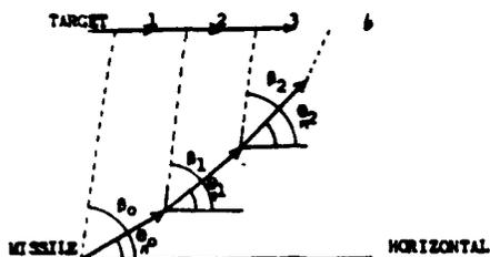
(d) Proportional. A course in which the rate of change of missile heading is directly proportional to the rate of rotation of the line of sight from the missile to target
