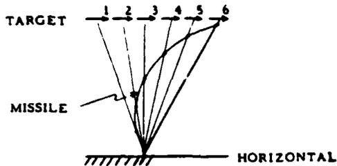
(a) Line of sight. Defined as a course in which the missile is guided so as to remain on the line joining the target and point of control.
