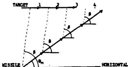
(c) Constant bearing. A course in which the line of sight from the missile to the target maintains a constant direction in space. If both missile and target speeds are constant, a collision course results
